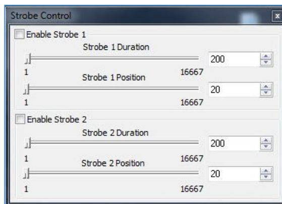
Figure 24: Strobe Control configuration screen.
