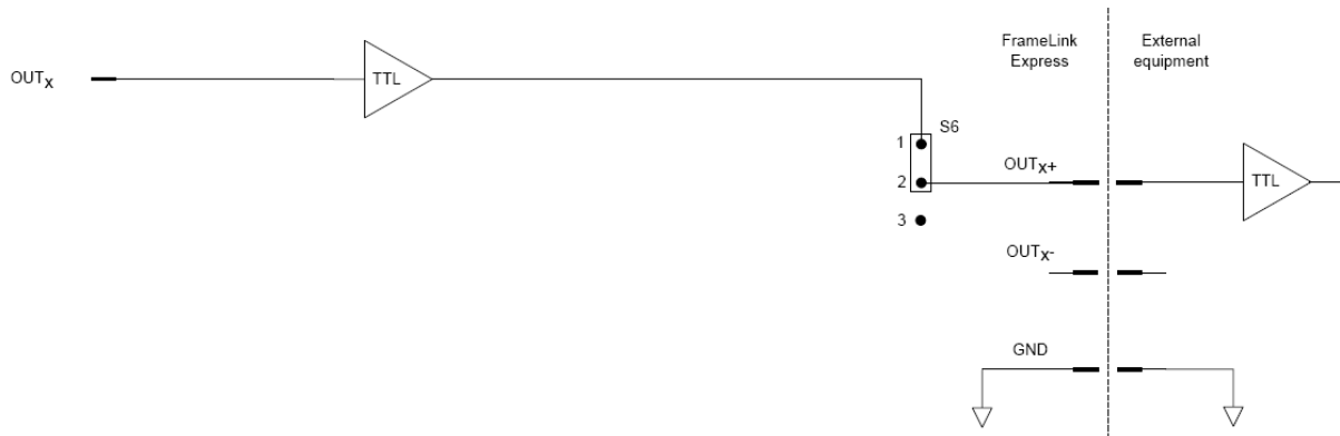
Figure E.11 – TTL Output Circuit
